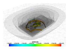
Simulations have been performed that consider the deformation of an initially intact caprock, caused by the depletion of an underlying reservoir during oil extraction. Deformation and flow are geomechanically modelled in three dimensions using a fully coupled poroelastic model, incorporating discrete fractures and faults in the caprock. Fractures are represented explicitly in an
